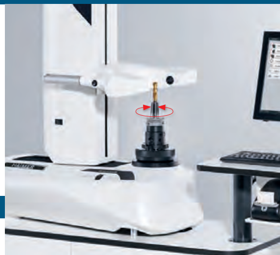
自动聚焦切削刃 Automatic focus on the cutting edge
