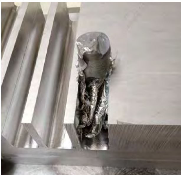
无Safe-Lock结构，刀具被拔出，工件报废 No pull out of the tool with Safe-Lock
