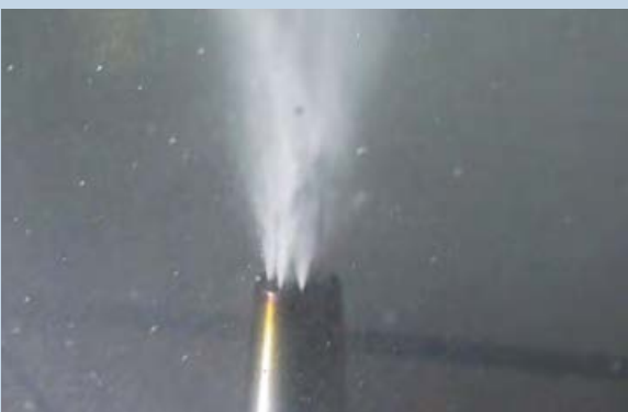
环绕冷却-直达刃口的有效冷却 Cool Flash – effective cooling at the cutting edges
