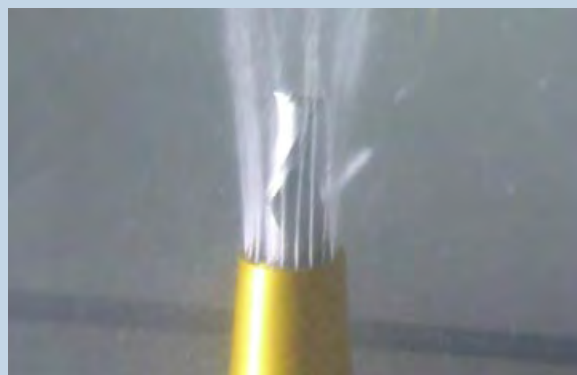
喷嘴冷却-无效冷却，冷却液不能到达切削刃 Slip-on sleeve with nozzles – ineffective cooling, coolant does not reach the cutting edges
