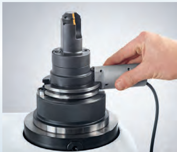
读写头的手动定位 Manual positioning of the read/write head
