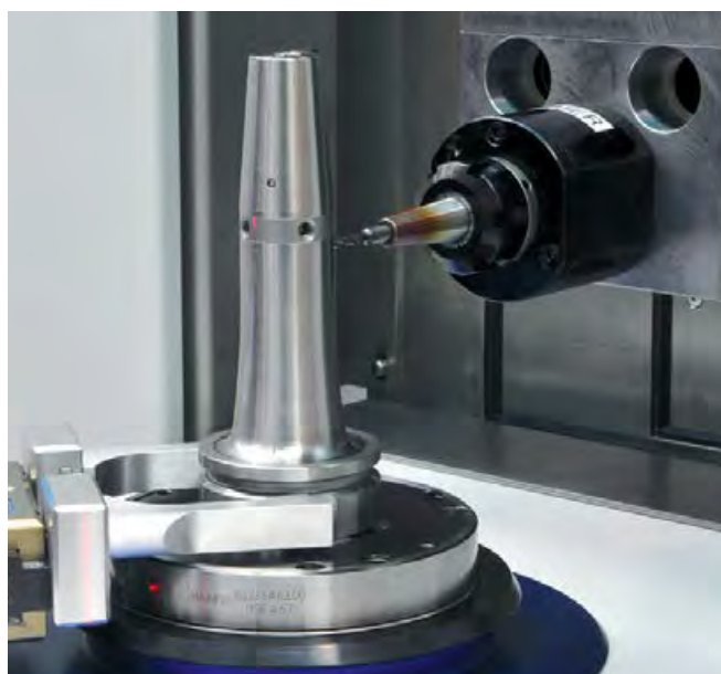
数控加工单元自动补偿不平衡量 Automated compensation of unbalance via CNC machining unit
