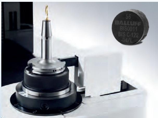
对刀仪测量刀具后, 数据传输到巴鲁夫的芯片内 After measuring the tool, the data is transferred to the Balluff data carrier
